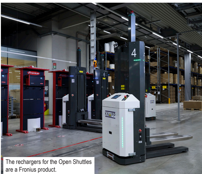
Efficient energy management means that the AMR automatically moves to the charging station when there are no immediate transport jobs.
