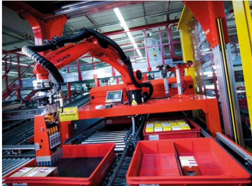
Man and machine share the workload in the warehouse of the future. The Pick-it-Easy Robot works at a rate of 300 picks per hour and therefore provides its human colleagues with considerable relief when it comes to carrying out strenuous work.
