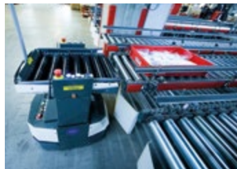
The Open Shuttles in the goods-in area avoid obstacles completely independently.
