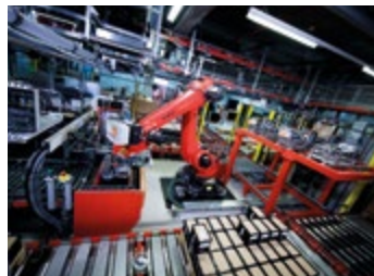
In addition to the 7 manual work stations for fast picking, a robot now also helps to relocate the articles for storage in the OSR Shuttle™.
