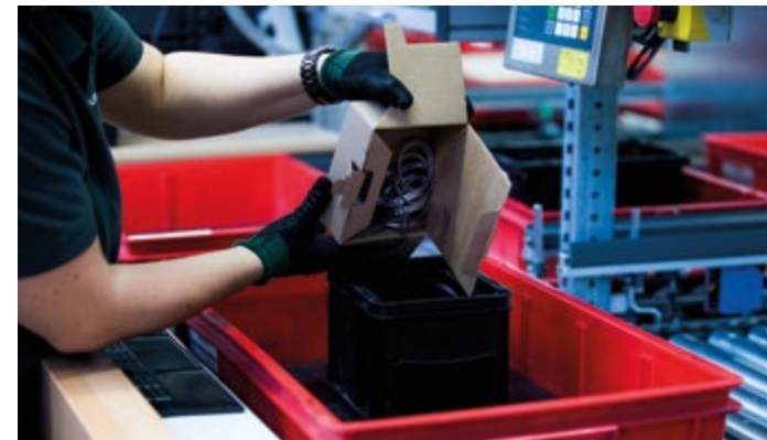
Container picking for supplying customers according to the Kanban principle takes place at 20 ergonomic Pick-it-Easy work stations.
