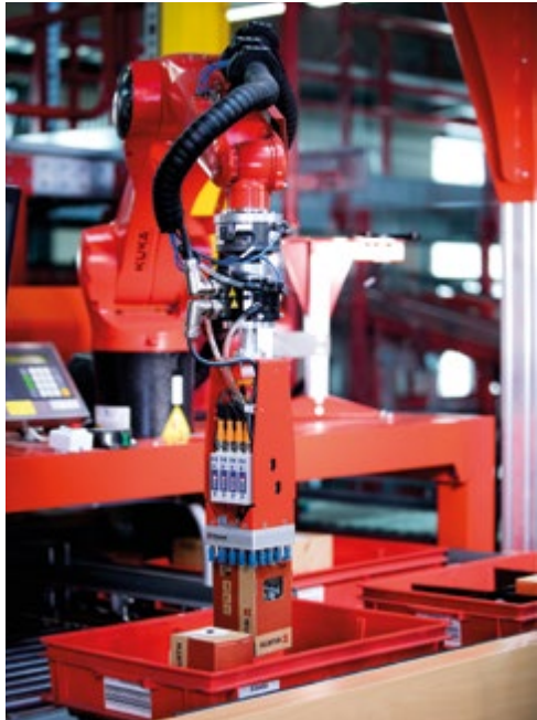
Man and machine share the workload in the warehouse of the future. The Pick-it-Easy Robot works at a rate of 300 picks per hour and therefore provides its human colleagues with considerable relief when it comes to carrying out strenuous work.
