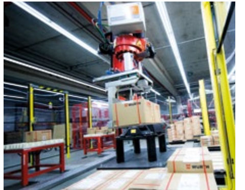
Another process is automated with a robot for palletizing cartons.
