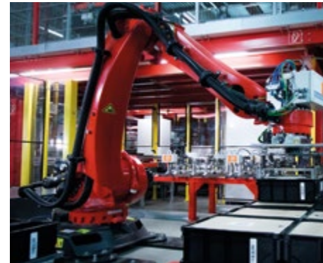
Small load carriers are placed on the shipping pallets in the right sequence fully automatically by two robots.
